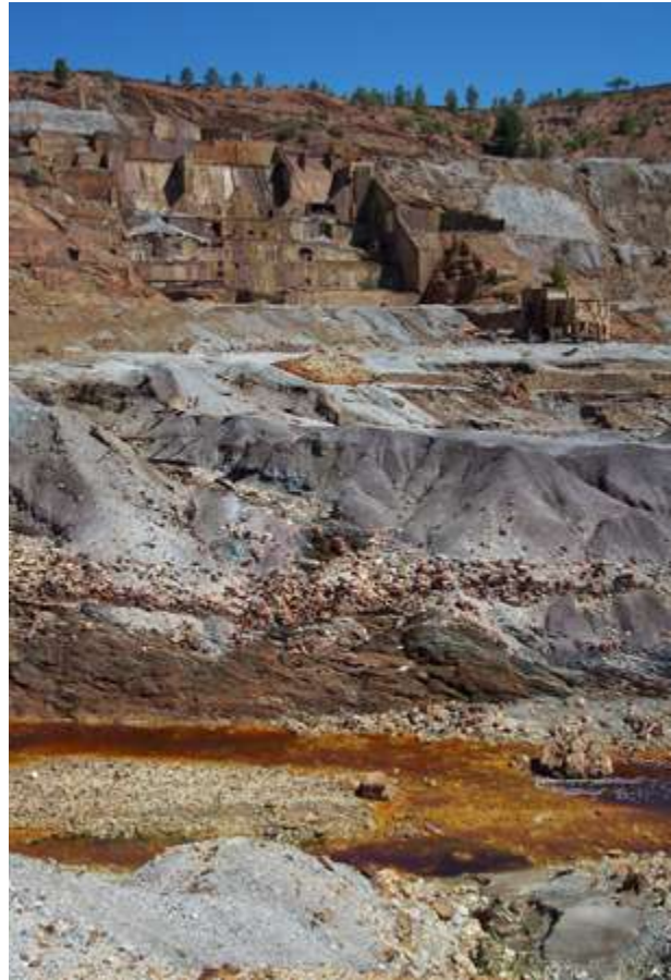
Figure 2.6: Mineral processing wastes and abandoned mining infrastructures by the Tinto River (Zarandas-Naya zone).
