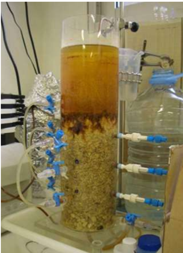
Figure 7.19: Column filled with reactive materials for the design of AMD treatment based on DAS technology. The flow is from top to bottom. Precipitates formed at the contact of the reactive material with AMD are visible.
