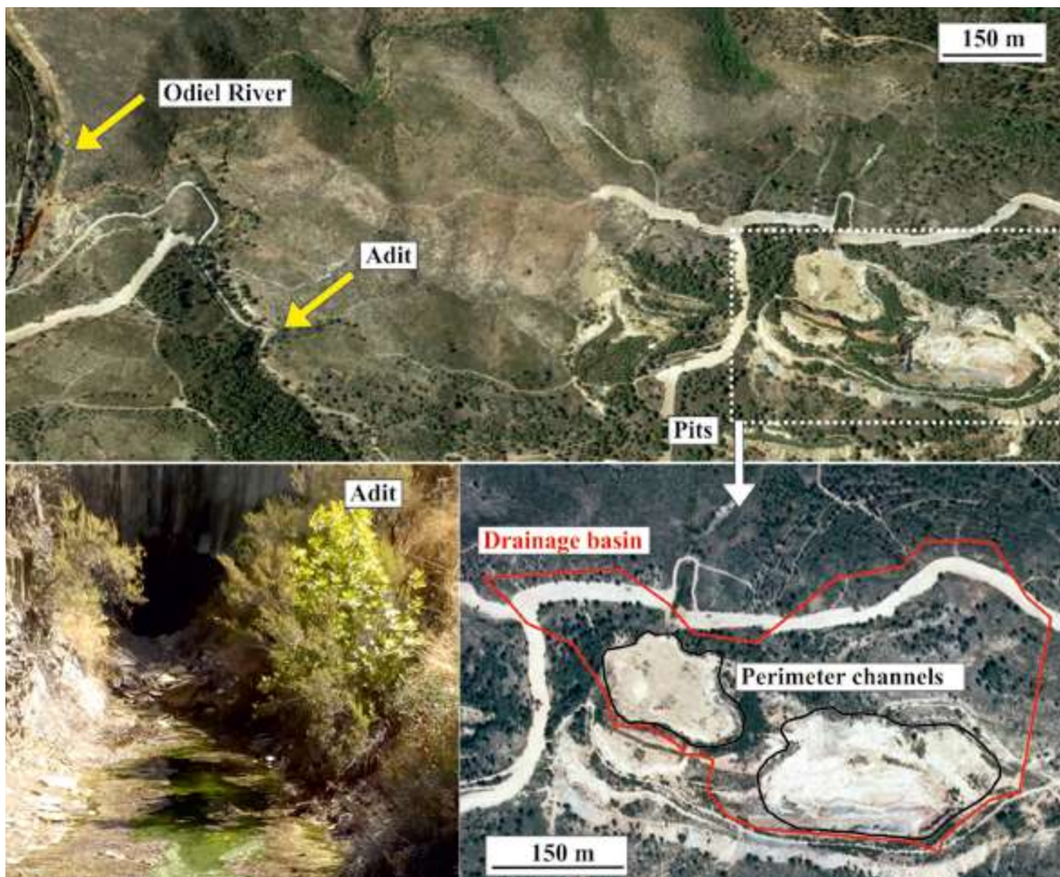
Figure 7.3: Aerial images and photo of Poderosa mine outflows, showing the drainage basin of open pits and the potential location of perimeter channels to reduce the AMD generation (aerial images from Google Earth).
