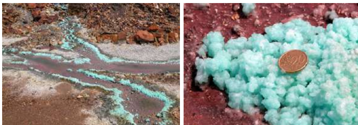
Figure 2.12: Photos of bluish evaporitic salts (mainly melanterite) on the margins of a leachate from the Riotinto mines (left) and a detail of the efflorescences (right).
