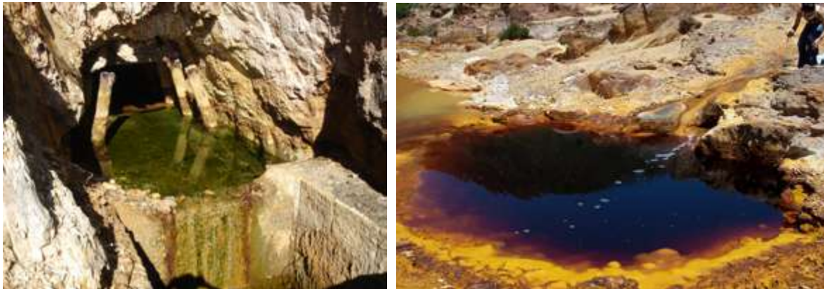
Figure 2.3: Photos of acidic drainages outflowing from Esperanza Mine, with high concentrations of \text{Fe}^{2+} (left) and drainages from Poderosa mine, with more oxidizing conditions and high concentration of \text{Fe}^{3+} (right).
