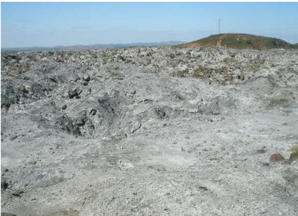
Figure 2.4: Sulfide dumps at Filón Sur (Tharsis mines). Rainfall waters infiltrate into the dump, leading to the oxidative dissolution of sulfides (note the small dissolution sinkholes) and the generation of highly pollutant drainages.
