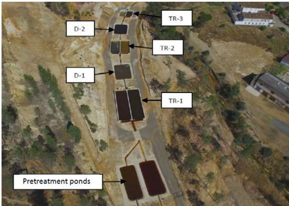
Figure 7.26: Aerial image of the different components forming the Concepción Mine (TR: reactive tanks; D: settling ponds).
