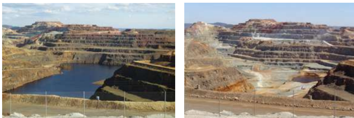
Figure 5.12: Left: Cerro Colorado pit lake in 2015, before the reopening of the Riotinto mine. Right: Cerro Colorado pit lake in 2017 after the pit lake water withdrawal.
