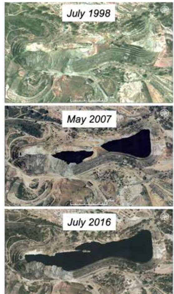
Figure 5.26: Orthophotographs showing the progressive flooding of La Zarza pit lake.
