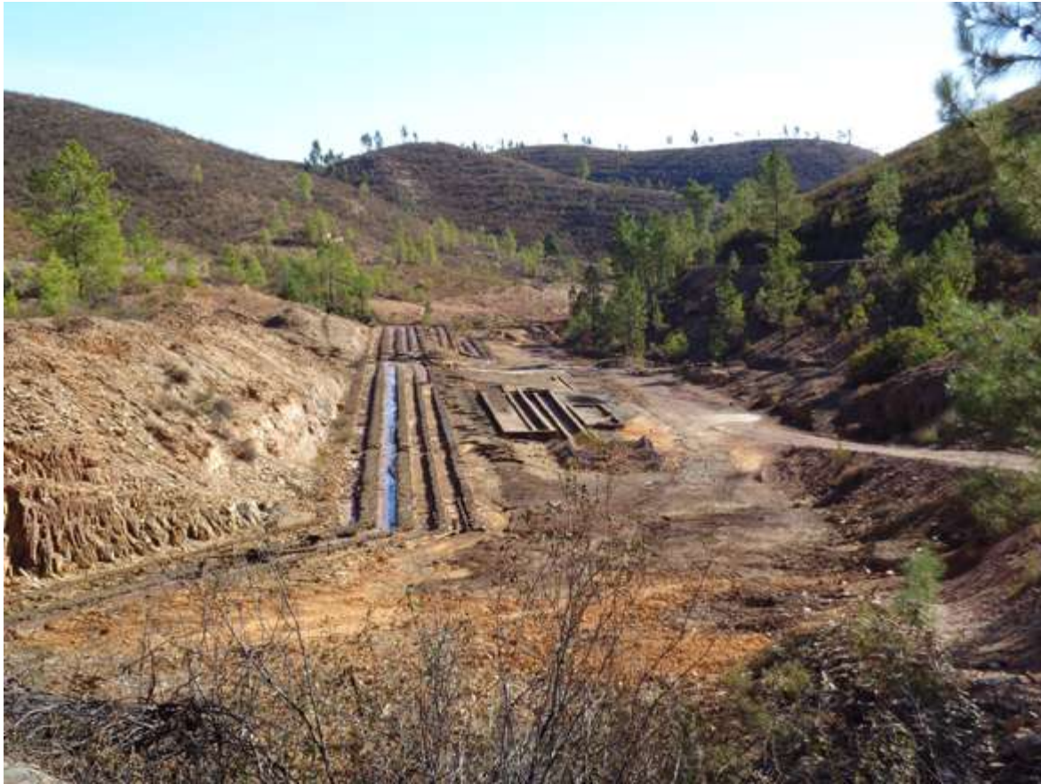
Figure 3.12: Channel system for copper cementation at La Zarza mine, which was in use until the 1960s.
