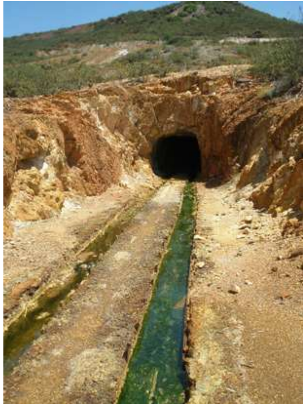
Figure 4.34: Greenish acidic leachates outflowing from La Sabina gallery (Tharsis mine), which are collected by the Valdeoscuro stream.
