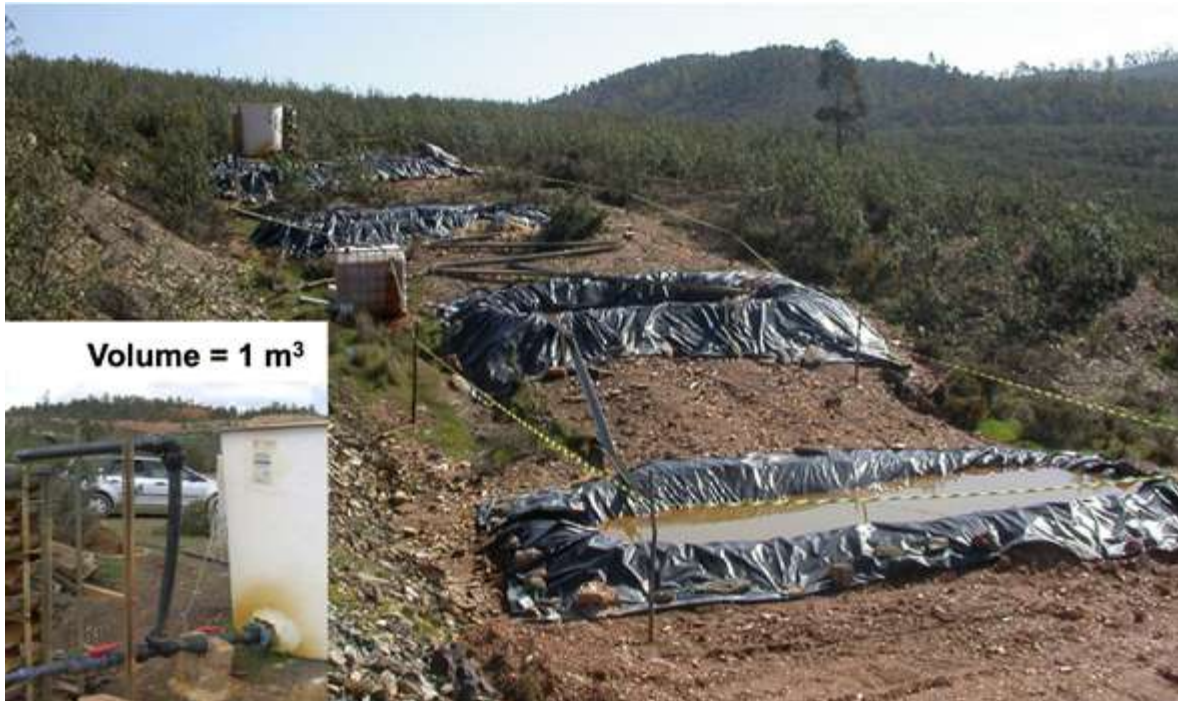
Figure 7.20: Pilot plant for AMD treatment based on DAS technology in Monte Romero mine.
