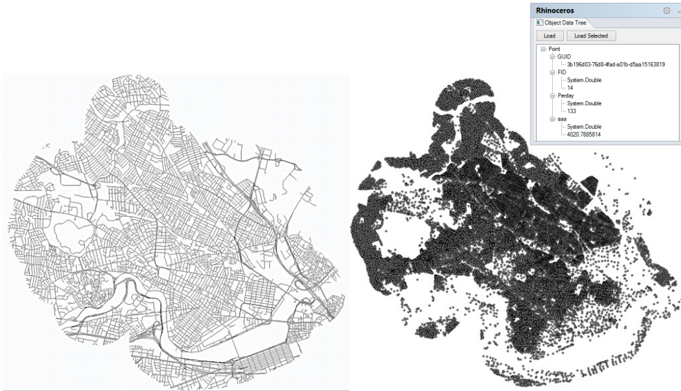
Figure 1. All UNA analyses require a network input, along which all trips are modeled, and point datasets to describe pedestrian origin and destinations. Each of these input elements can contain attribute information that can be used as 'weights' in analyses.
