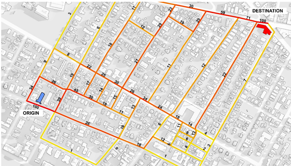
Figure 3. Stochastic route assignment for 75 trips, which allocates an equal probability to all routes that are up to 20% longer than the shortest available path.
