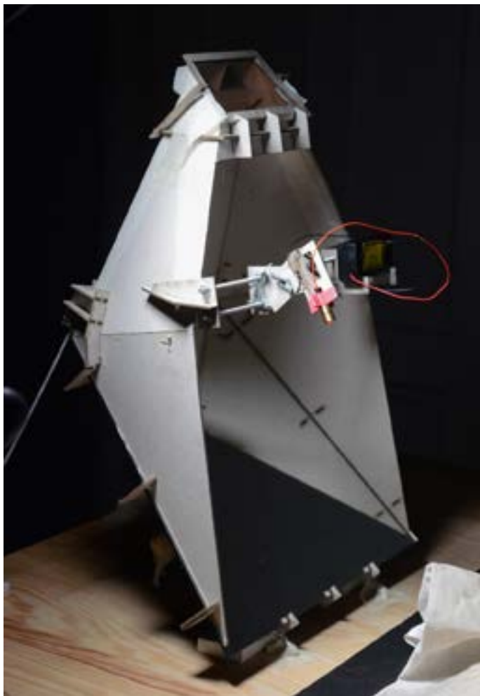
Figure 1. Stereoscopic camera lucida inspired by the Wheatstone Stereoscope, equipped with a line laser, which casts a cutting plane onto the object of observation, a folded cloth.
