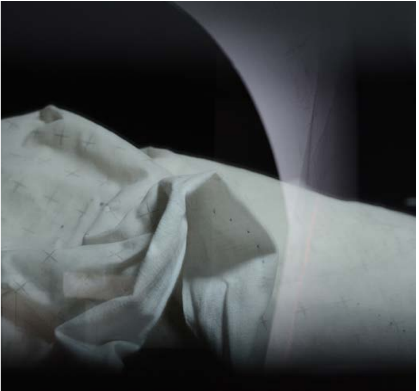
Figure 4. A line laser casts a cutting plane onto the object of observation, a folded cloth, where the folded drawing paper is positioned to trace the section.
